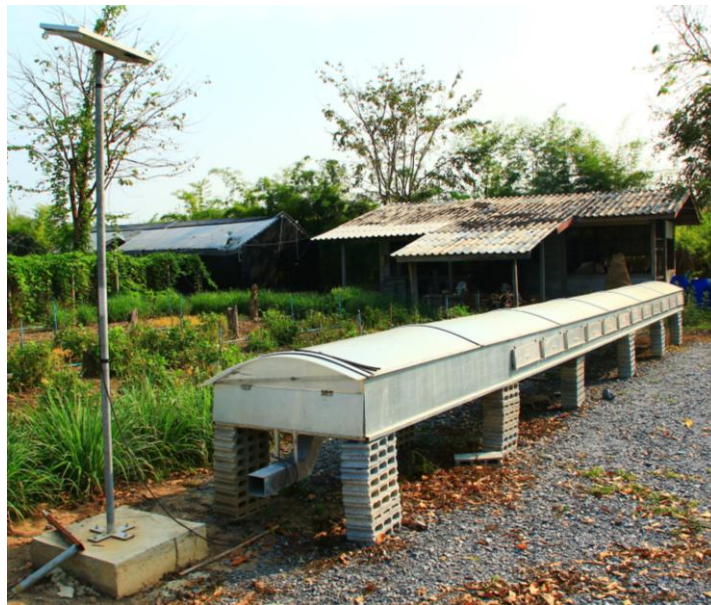
Fig. 2. Illustration of parabolic-shaped solar tunnel dryer
