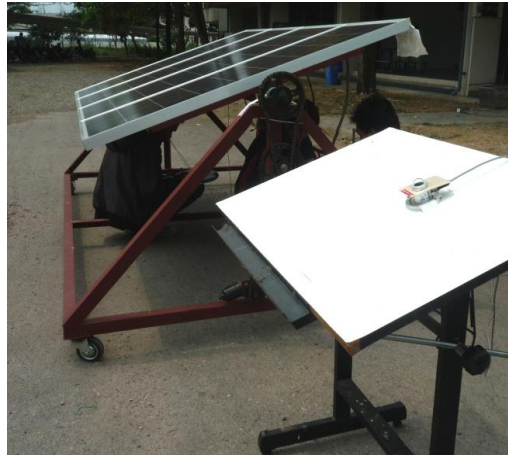
Fig. 2. Setting PV module for tilt angle experiments
