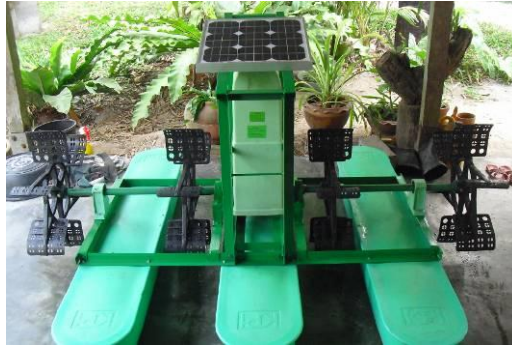
Fig. 12. The prototype of a solar water turbine
