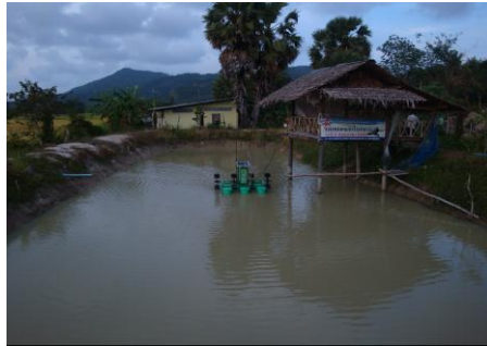
Fig. 13. The prototype of a solar water turbine in the 5*10 meters catfish pond
