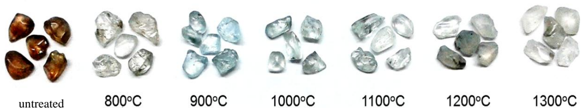
Fig. 1. Visual appearances of Cambodia zircon before and after heat treatment under CO 2 atmosphere at various temperatures for 6 hours
