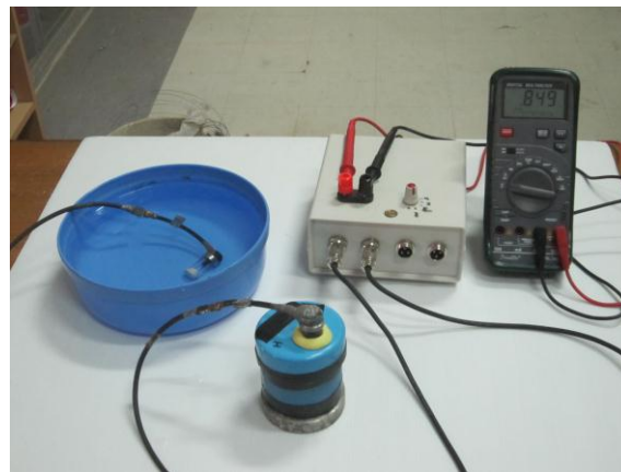
Fig. 1. Experimental set up for suction-monitoring
